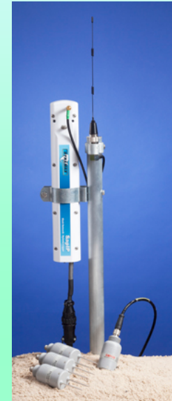
Soil Moisture Node w/ Soil Moisture Profile
