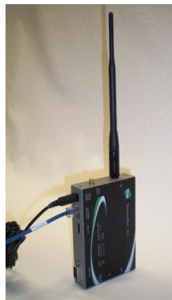
Internet Gateway – Base Station
