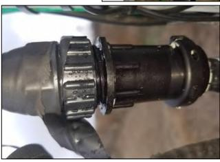
With the seal leaking with water on the white rescue seal after 6 months, and there is one broken wire.
