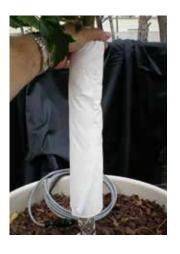
12) Install bubble shield on the stem below the sensor with tape. Try to insulate at least two sensor lengths or more of stem below where the sensor is installed.
