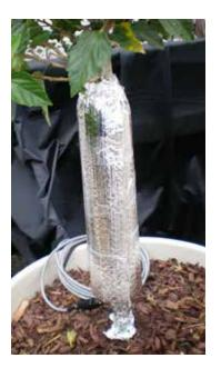
13) Install bubble shield around the entire sensor and tape in place, especially at the top. Leave the bottom of the bubble wrap un-taped for ventilation.
